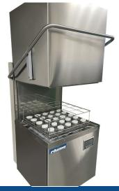
415V Power supply Total power 7.1KW Total current 16 Amp Wash tank capacity 15 ltrs Water consumption (wash & rinse cycle) 15 Itrs 75°C Rinsing temp (approx) 500mm x 500mm Rack size Tallest washable item 42 cm Weight (empty) 92 kg 3/4" hose Water connection (Hot\*) \*Connect to hot water for optimum performance
