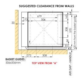
Note: Dimensions shown are a guide only. Benching design/measurements may vary depending on individual site requirements. Rhima suggests final bench design is done with washer in place.
